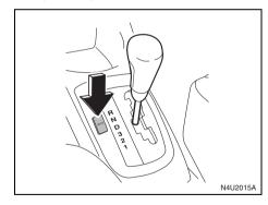
Press the HOLD button on the shift lever to turn on the HOLD mode.
